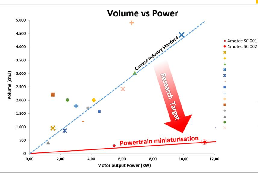
The competitor analysis for DC-AC inverters up to 10KW (cont.) considers an average available battery voltage of 50,4 V
