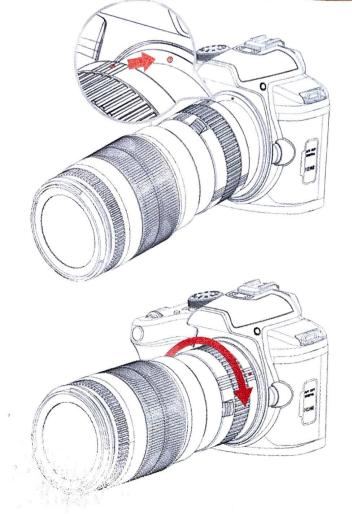
4. To remove the tube with lens from the camera, press the lens release button on the camera and rotate the tube counterclockwise to release them. Then press the black button on the tube while turning it counterclockwise to remove it from the lens.
