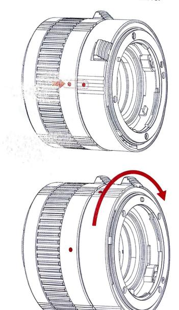
3. Switch the camera to OFF, then position the tube into the camera's lens mount with the red marking aligning with the one on the camera, then twist the tube with lens clockwise until it clocks into place.
