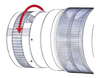
2. When using more than one extension tube, combine them with one tube's rear red marking aligning with another tube's front one, and then rotate the tube in your right hand clockwise until it locks into place. Now you can mount them to your lens as mentioned above.
