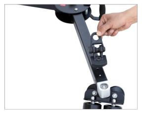
• Insert the screw as shown to attach the foot clamp with dolly and tighten with the help of allen key.
