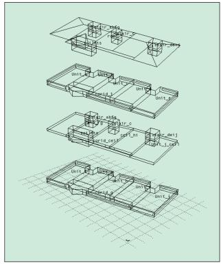
Exploded view of geometric model in ESP-r.
