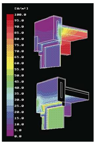
3D display of thermal condition simulation in new construction element.
