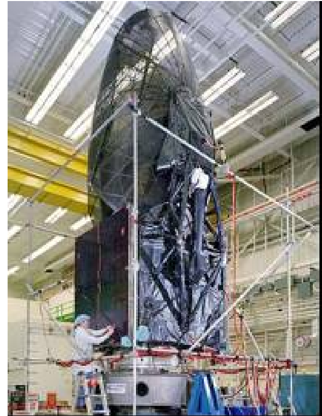
Hughes SBA (a) one stowed another deployed, (b) vibration test on TDRS-H (two SBAs are stowed on the top of the satellite)
