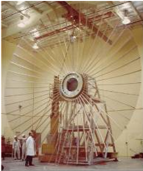
9.1 m WRA launched in 1974 with the Applications Technology Satellite 6
