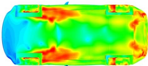
(a) Simulated sound pressure distribution on the underbody of a vehicle [O. Szulc, Siemens Industry Software & IMP Polish Academy of Sciences]
