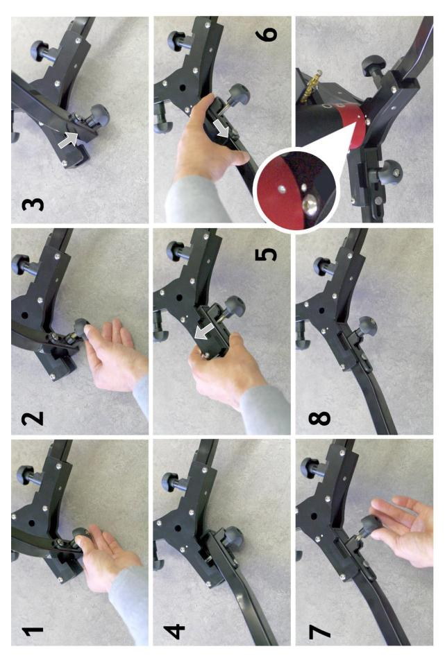
Note that the Base Piece (21) of the column has a white indication point that should be pointed at the white indication point on the dolly housing (15). This position makes the Pedestal with Spider ideal foldable.
