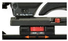
Turn knob to left to unlock and to the right to lock. Remove the cameras lens shade. Position camera lens within 1/2" from glass.
