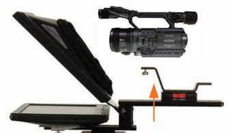
The camera should be mounted with it's lens vertically centered in the beamsplitter. Choose the side of the riser that puts the camera in this position. Secure camera to riser with attached camera screw. When camera is mounted slide it gently forward until lens is one inch behind glass beamsplitter. Rotate red knob in "lock" direction to secure camera in place.
