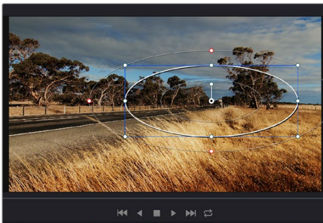
Power windows let you make secondary corrections to specific parts of your image
