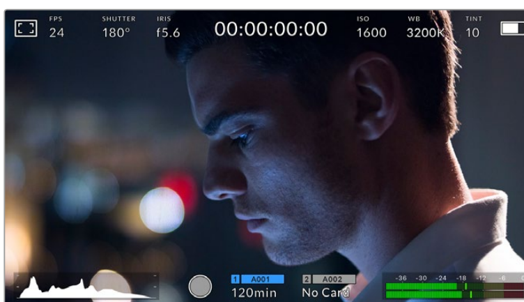
Your URSA Mini's LCD touchscreen has a comprehensive head up display and gives you easy access to your camera's most used settings
