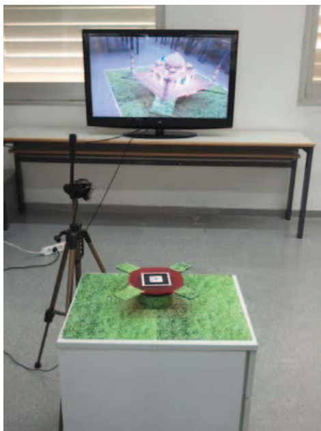
Figure 1: Table with the marker on the rotator support, camera and autostereoscopic display.
