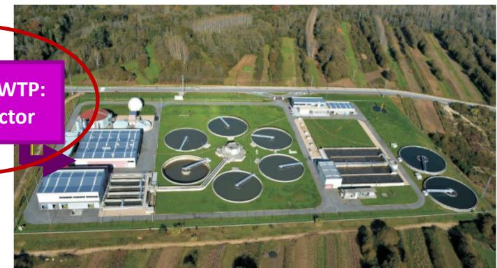
The PN-AMX reactor is placed in the reject line in the WWTP
