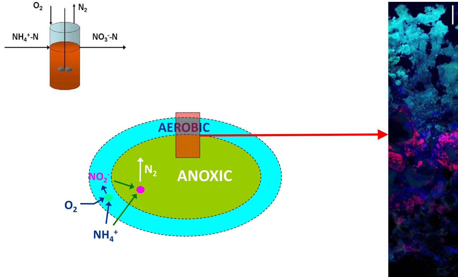
The structure of the granules allows for an external aerobic and an internal anoxic layer
