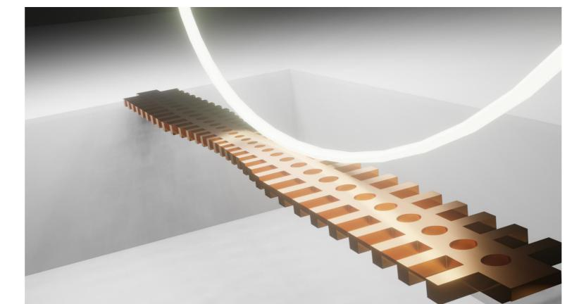
In this context, we propose and optomechanical demonstrate an simultaneously crystal cavity that holds several confined mechanical modes as a function of the cavity design. By adding transition cells to the cavity, new GHz mechanical modes appear.
