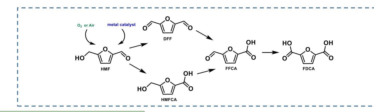
The use of catalysts based on Ru nanoparticles allows to obtain high yields and selectivity of DFF.
