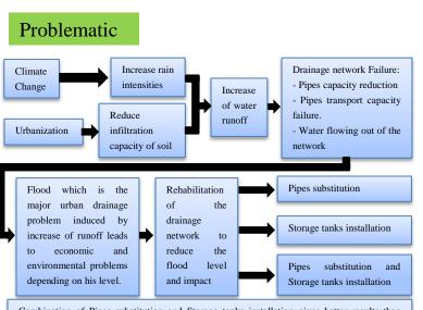
Combination of Pipes substitution and Storage tanks installation gives better results than pipes substitution or storage tanks installation applied separately. The problem is the fact that the implementation of this option is numerically costly and the question is: How can we overcome this situation?
