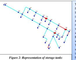
The nodes in red on figure 2 represent the location where should be installed storage tanks and the conduits in red represent the locations where pipes should be substitute to reduce Floods according to the scenario 5 presented in Table1. A total of 3 storage tanks to be installed and 4 pipes to substituted be to rehabilitate the network.
