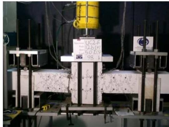
**Fig. 6.** Specimen #3 at 5% drift
