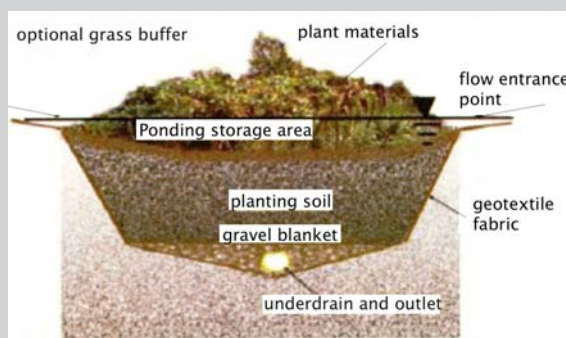
Figure 36: Diagram of a bioretention area
