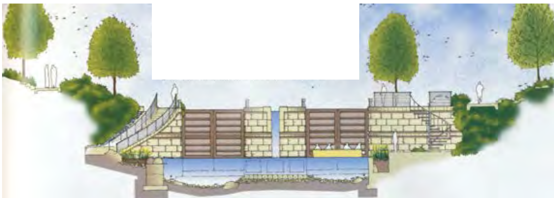
Figure 38. San Antonio River Walk. North Reach at Brooklyn Avenue. Damming the North Reach will enable passenger barges from the existing river walk to navigate farther north. Bottom, planted crib walls allow for vegetation and bank stabilization while cobblestones line the river bottom, promoting the growth of organisms and a healthier river ecosystem.
