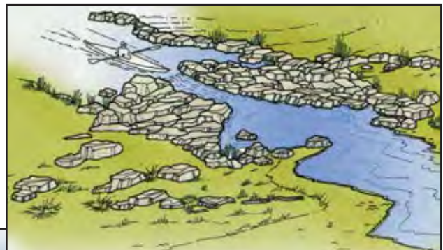
Figure 40. San Antonio River Walk. South Reach Plan. Grade Control Structures, in the form of indigenous limestone weirs, span the south reach, controlling water flow so that it does not scour and erode the bottom of the river. The weirs are designed to allow passage through a narrow opening, a nod to local canoe enthusiasts.
