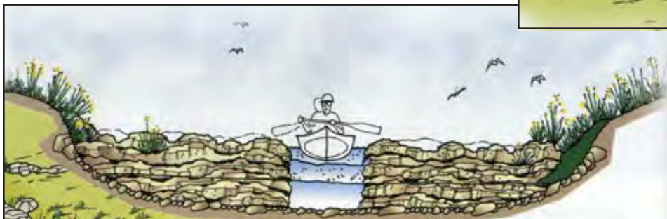
Figure 40. San Antonio River Walk. South Reach Plan. Grade Control Structures, in the form of indigenous limestone weirs, span the south reach, controlling water flow so that it does not scour and erode the bottom of the river. The weirs are designed to allow passage through a narrow opening, a nod to local canoe enthusiasts.
