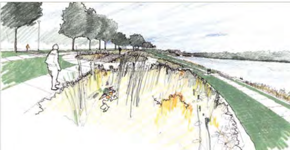
Figure 24. ATF, 2006. The Garden and Overlook at 22n Ave. N. Rain gardens will be used to treat stormwater runoff, stable slope, and remove sediments.
