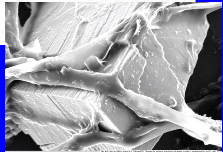
FIG. 4.6 Fungi attacking a crystal of Galena (PbS). Observe the mode of attachment of fungal hyphae to mineral surface at 90°. (X3)
